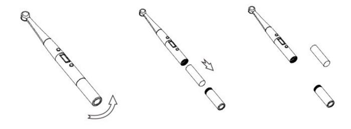
4.4 When device needs to charge, firstly insert the DC connector of the power adapter into the charging jack marked on the charger cradle, and then connect the power adapter to the AC 100V–240 V electricity network, and then place the host in the center of the charger cradle to charge.
